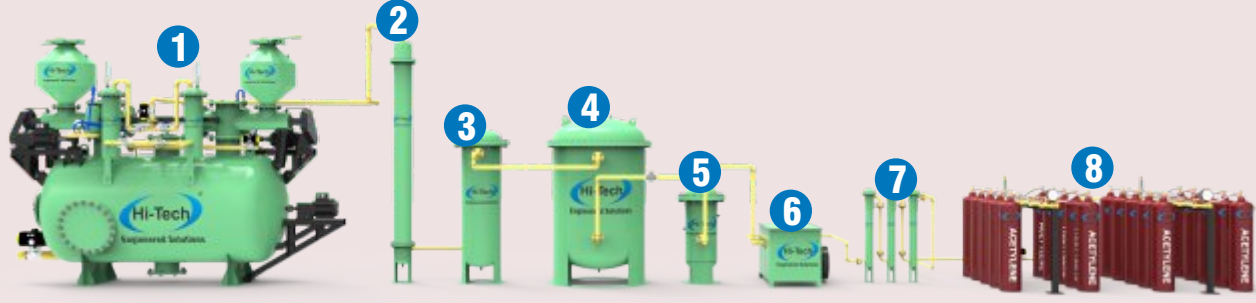
Typical Process Flow Diagram for Acetylene Cylinder Filling
